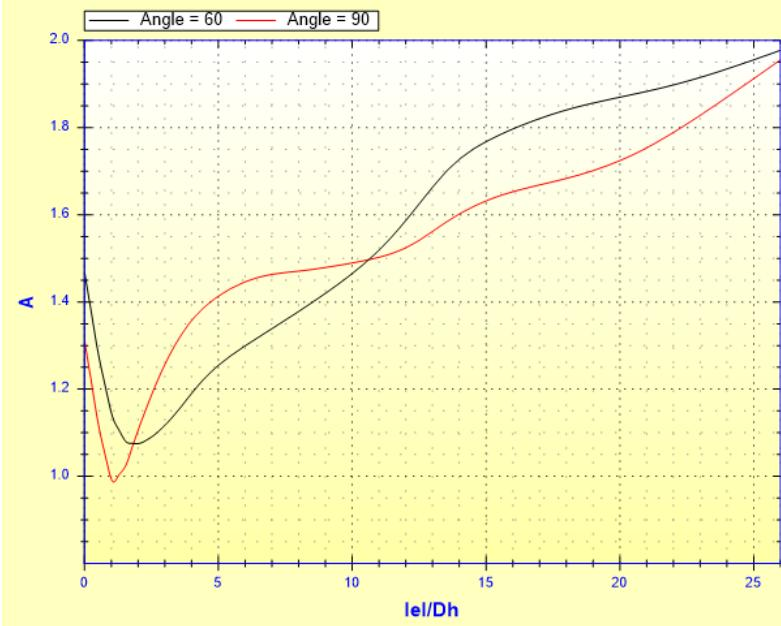
Total pressure loss coefficient (based on the mean velocity in the bends):
