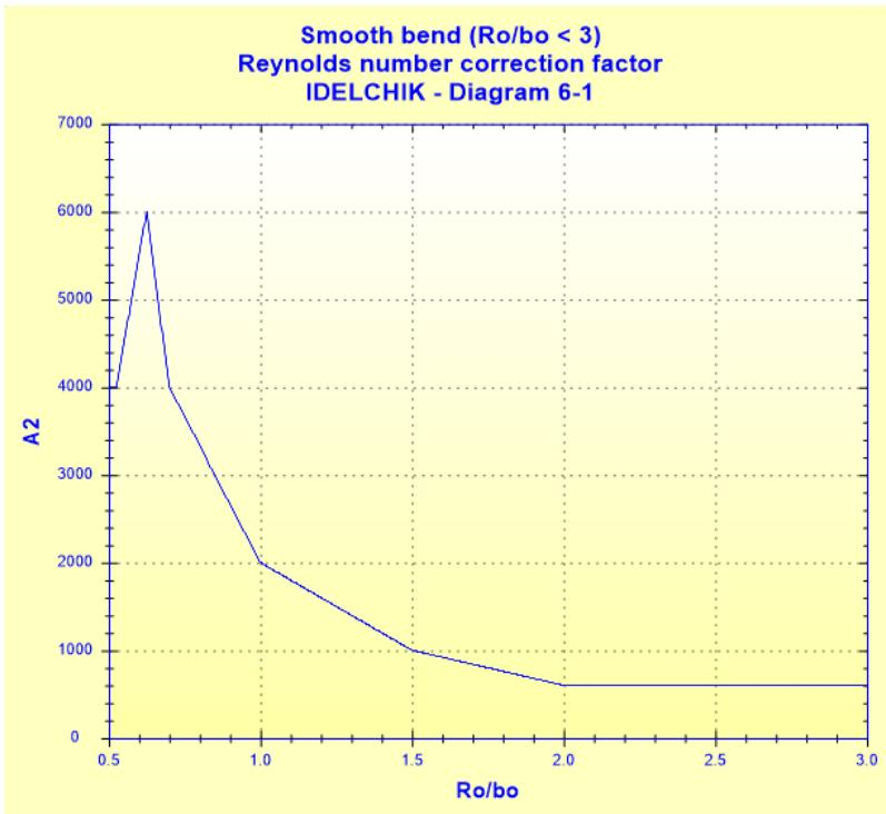
Pressure loss coefficient (without friction):
