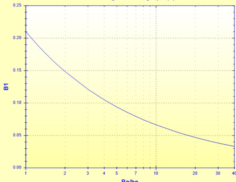
**Coefficient of effect of the relative elongation of the cross section:**
