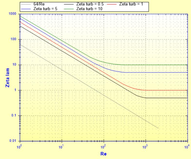
Total pressure loss coefficient (based on the mean velocity in the bend):
