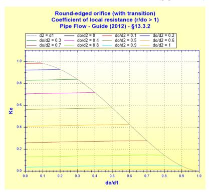
Total pressure loss coefficient (based on the major pipe velocity):
