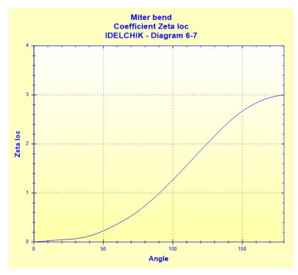
Total pressure loss coefficient (based on the mean velocity in the bend):
