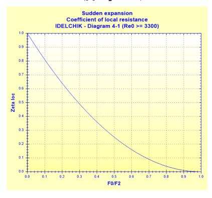
Total pressure loss coefficient (based on mean velocity in minor diameter):
