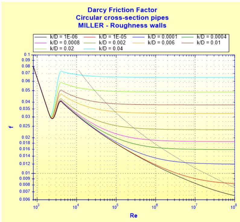
Friction pressure loss coefficient:
