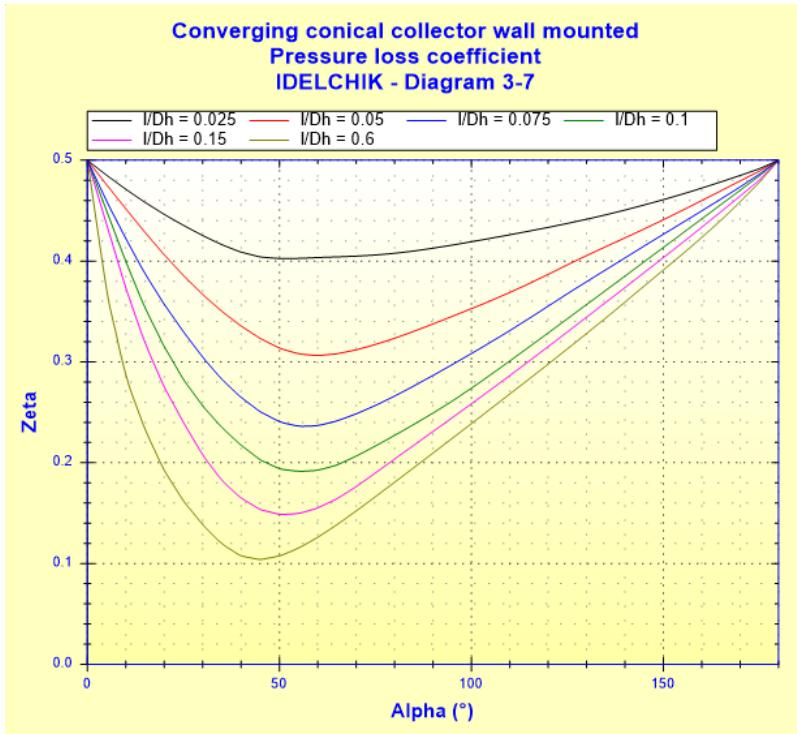
Total pressure loss coefficient (based on mean velocity in pipe):
