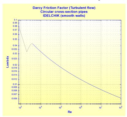
■ critical flow regime (2000 < Re < 4000): interpolation between laminar and turbulent flows
