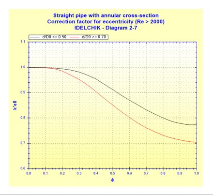
Darcy friction factor for annular cross-section:
