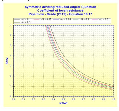
Pressure loss coefficient of the right branch:
