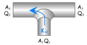
Coefficient based on mean velocity in the common branch:
