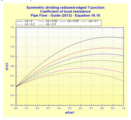
Coefficient based on mean velocity in the left branch:
